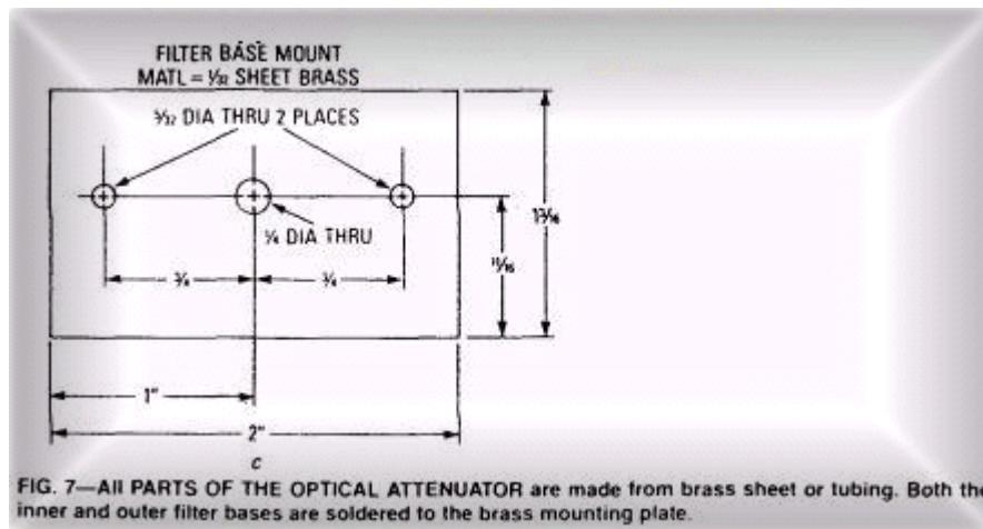
When both filters are in place, rotation of the large-diameter filter-mount will cause a gradual decrease in light transmission (to almost total blockage within 90 degrees of rotation), which allows the receiver to be used over a wide range of light intensities without swamping the photo detector.
