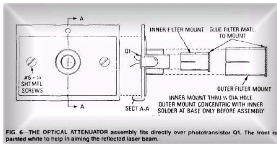
Figure 6 shows how it's installed over Q1: Fig. 7 shows the individual details for each component in the assembly.
