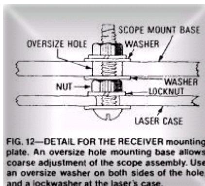
FIG. 12—DETAIL FOR THE RECEIVER mounting plate. An oversize hole mounting base allows coarse adjustment of the scope assembly. Use an oversize washer on both sides of the hole, and a lockwasher at the laser's case.
