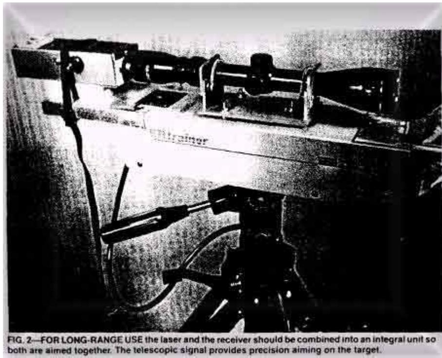
FIG. 2—FOR LONG-RANGE USE the laser and the receiver should be combined into an integral unit so both are aimed together. The telescopic signal provides precision aiming on the target.
