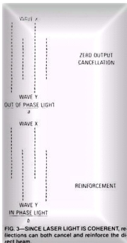
As shown in Fig. 3-a, the beams cancel each other when out of phase (destructive interference). As shown in Fig. 3-b, the beams are additive when in phase (constructive interference). It is the interference between the beams that enables the movement of any reflecting surface to be sensed by a device called an interferometer.
