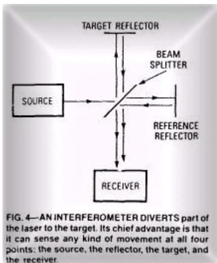
**FIG. 4—AN INTERFEROMETER DIVERTS** part of the laser to the target. Its chief advantage is that it can sense any kind of movement at all four points: the source, the reflector, the target, and the receiver.
